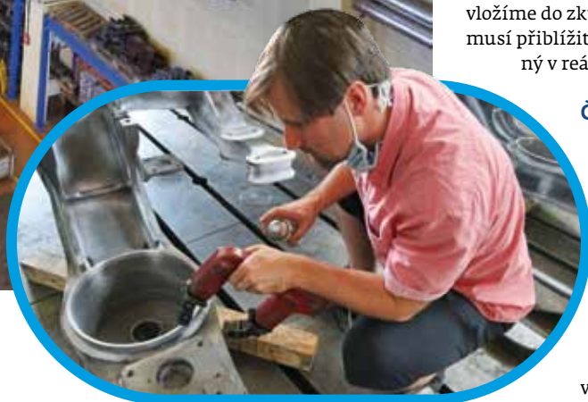
Provádění NDT (nondestructive testing) metoda MT (magnetic particle testing)
